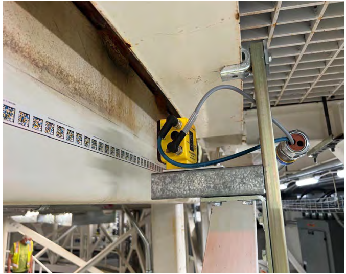
Figure 3.20. Enclosure azimuth with new barcode encoder and read head.
