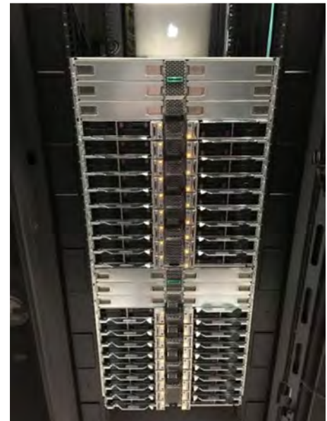
Figure 5-1. One rack of the first DKIST Level-2 1296 Core Cluster (36 nodes of 18 x 2 cores with Xeon 6150 2.7 Ghz processors, 192 Gb/node, interconnected with Infiniband).
