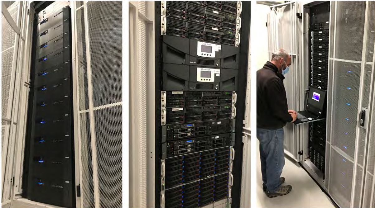
Figure 4-9. (left) The 1.5PB primary data storage cluster, (middle) the tape robots and auxiliary data storage, and (right) a software engineer at the console in the pipeline processing rack. Courtesy of N. Oien.
