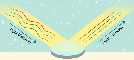
As part of the Adaptive Optics System, the Deformable Mirror has 1,600 actuators that will adjust the mirror's surface in real-time, at about:
