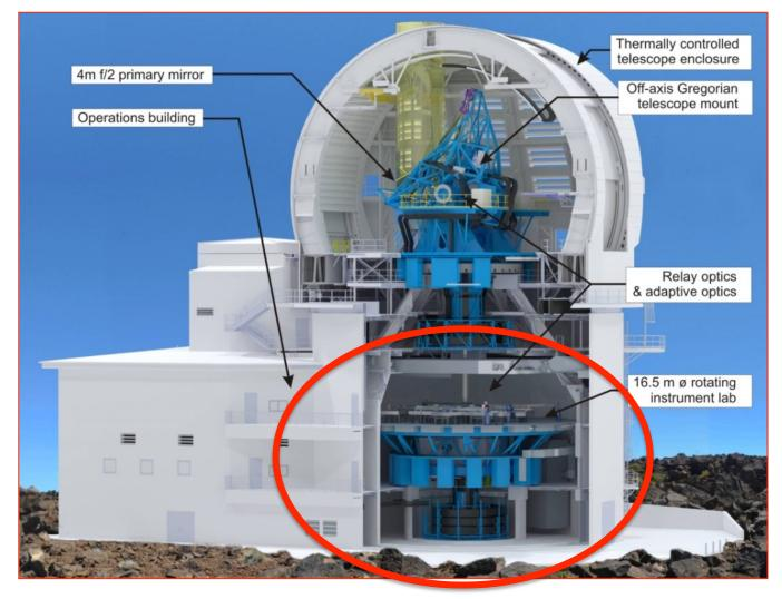
The Coude' lab ROTATES during the day to keep constant the solar image orientation on the scientific instruments
