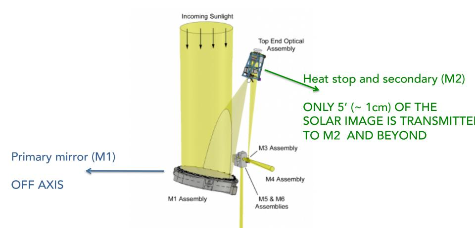
The assembly and control of the heat stop mechanism is much simpler, & safer, with an off axis!
