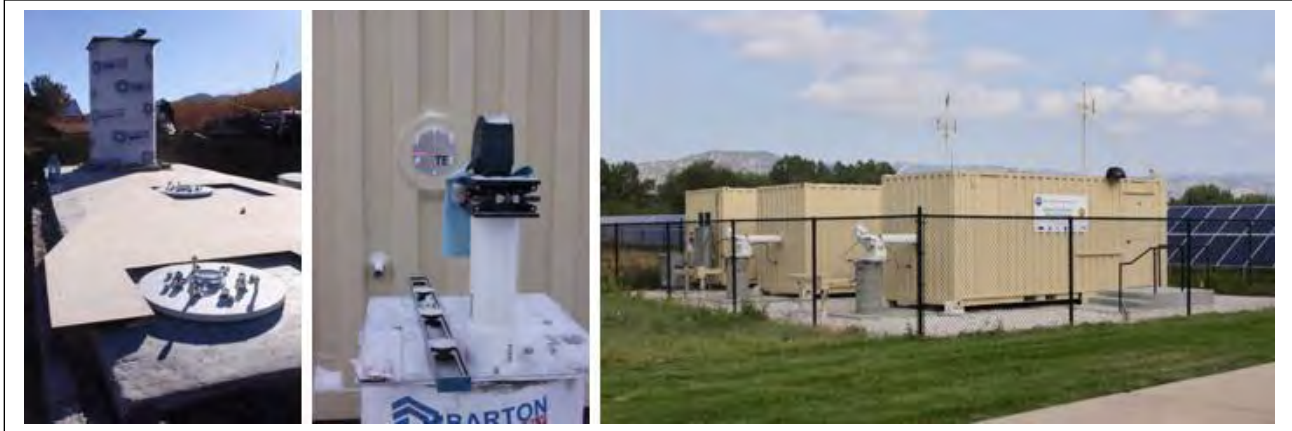
Figure 6-6. Alignment of the turret with the instrument mounting plates (left) and enclosure (middle). Completed GONG engineering site in Boulder (right).
