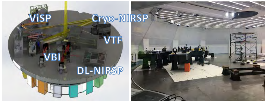
Figure 5-29. Left: Layout of the five first light instruments on the Coudé platform. Right: April 17, 2019 state of the Coudé platform showing the VBI and WFC tables.
