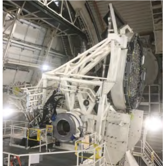
Figure 4-2. The telescope mount with the coated primary mirror (M1) installed and ready for first night-sky pointing tests. Photo by Heather Marshall.
