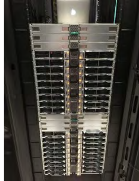
Figure 7-1. One rack of the first DKIST Level-2 1296 Core Cluster (36 nodes of 18 x 2 cores with Xeon 6150 2.7 Ghz processors, 192 Gb/node, interconnected with Infiniband).
