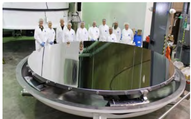
Figure 4-1. The DKIST mirror coating team with the freshly-aluminized primary mirror. Photo by Erik Starman.
