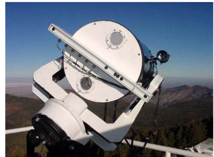
Fig 13. The ATST seeing monitor. Visible are the two circular apertures for the S-DIMM, the linear array of six scintillometers for the SHABAR, and a Meade telescope.
