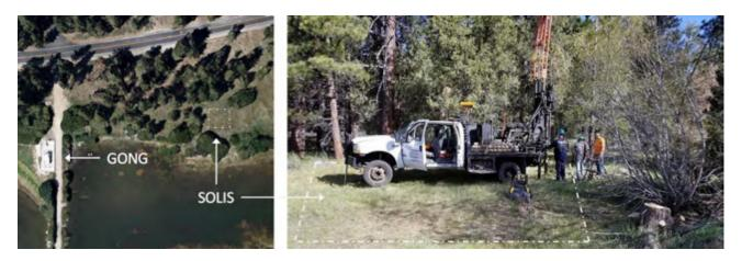
**Figure 6.2-1.** The aerial view (left) of Big Bear Solar Observatory indicates the future location of SOLIS relative to the existing GONG site. The ground view (right) of the SOLIS site shows the soil bore testing performed prior to construction.
