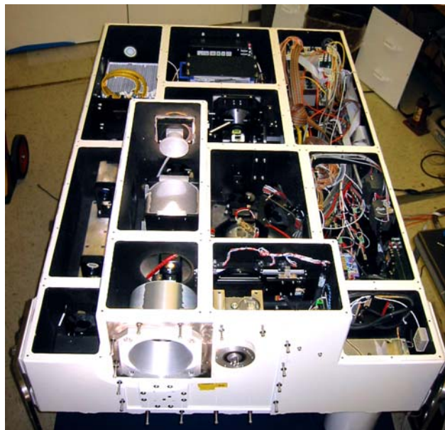
Figure 5. The FDP in its assembly and test configuration. Sunlight is fed to it by a rooftop heliostat. The objective lens is in the shiny cylinder at the bottom. The pupil of the instrument is a fast tip-tilt mirror at the far end of the upper bay. The 1083-nm filter is in the white cylinder just below the fast mirror. The left-hand bays contain the guider sensor and feed optics, and the right hand bays house the electronics for the cameras, temperature controllers and mechanism controllers.
