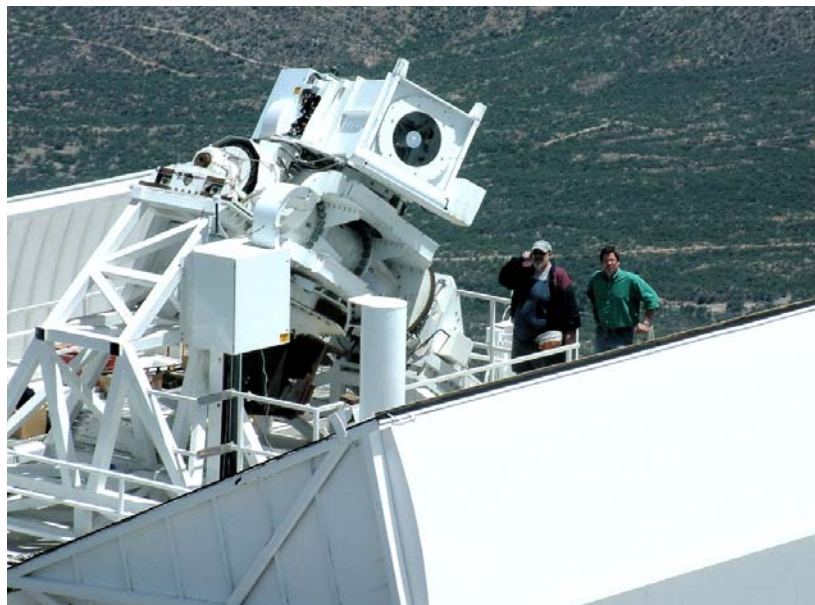
Figure 2. The SOLIS mount is installed on top of the old Vacuum Telescope Tower located on Kitt Peak. The VSM is the box-like structure on top with its entrance window exposed. A 50-cm aperture telescope occupies the near half of the box and a spectrograph the distant half. The entire instrument is filled with helium for thermal and seeing control.
