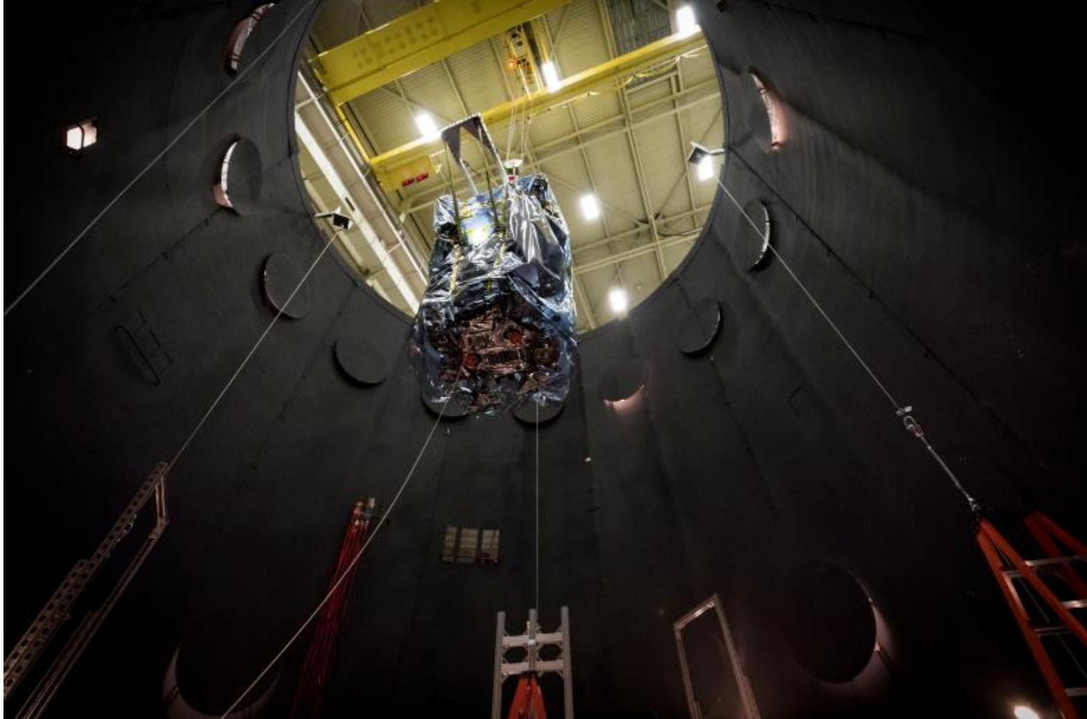
Flight Observatory successfully lifted and installed in the SES Chamber
