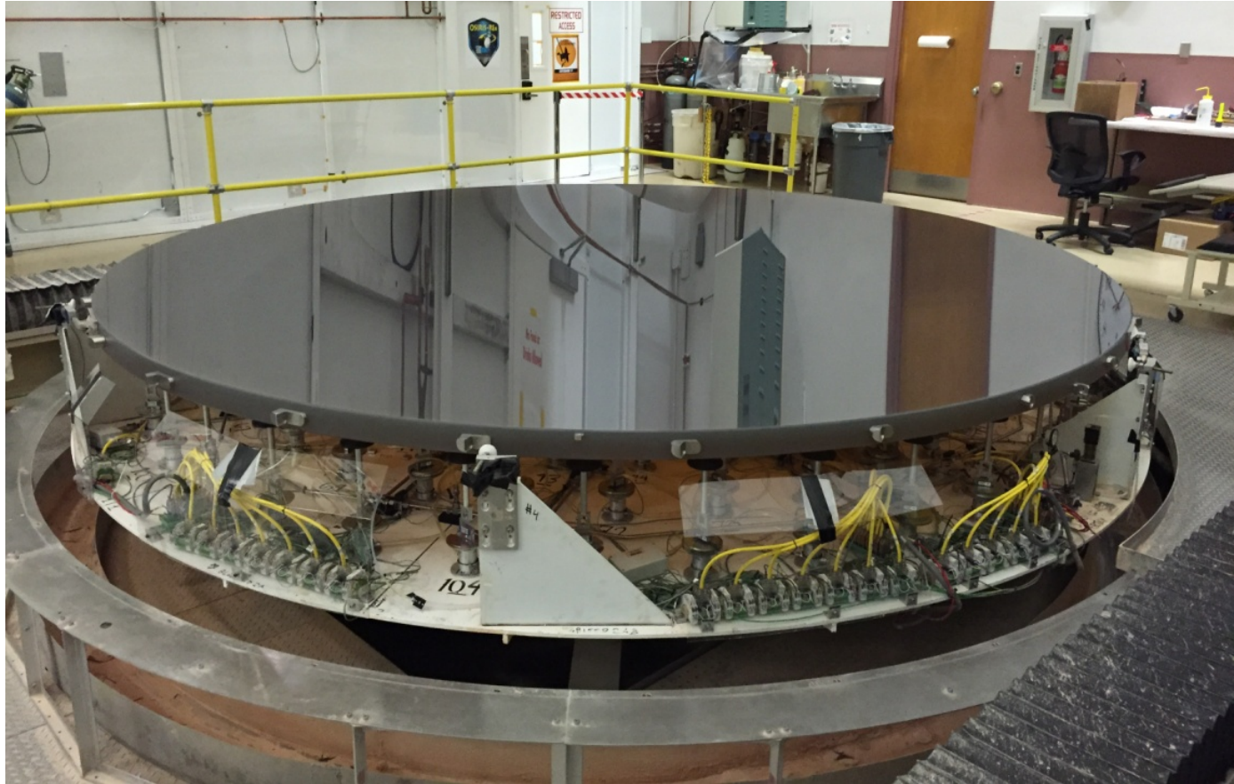
High-grade polished M1 ( \sim 1 nm)
